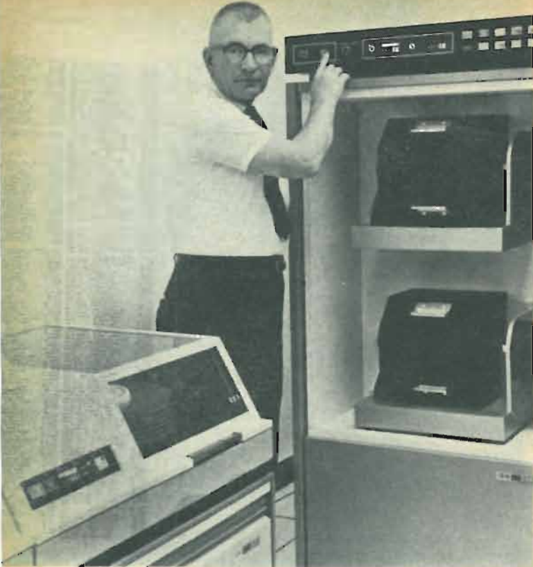
Fig. 1. New electronic photocomposing unit, controlled by an IBM System/360 computer, can set a newspaper page in ten seconds and a full-length novel in approximately ten minutes.
